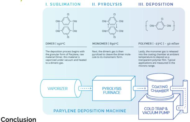
Dexter began developing it's in house BarrierMax 1 Parylene C coating process in 2018 and tailored its formulation to optimize performance on NdFeB magnets. Process variables were systematically tested and adjusted through a series of rigorous accelerated life and adhesion tests which included:
