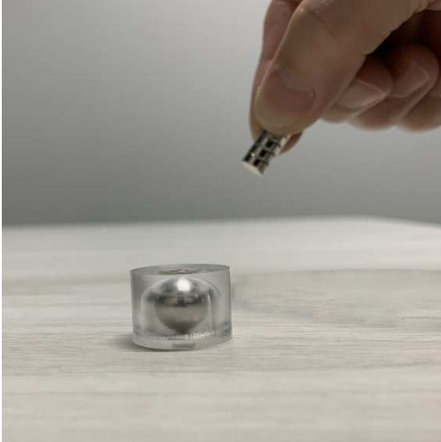
Fig. 6. Prototype of MRI-conditional implant magnet and reaction to homing magnet
