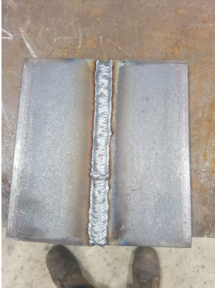
PHOTO OF MIG (WELDING)
